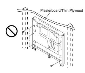
The Wall Mounting Unit should be mounted to a wall that can adequately hold the total weight of the plasma display and the Wall Mounting Unit over a long period of time and which can adequately withstand earthquakes, conceivable vibrations, and other external forces.
